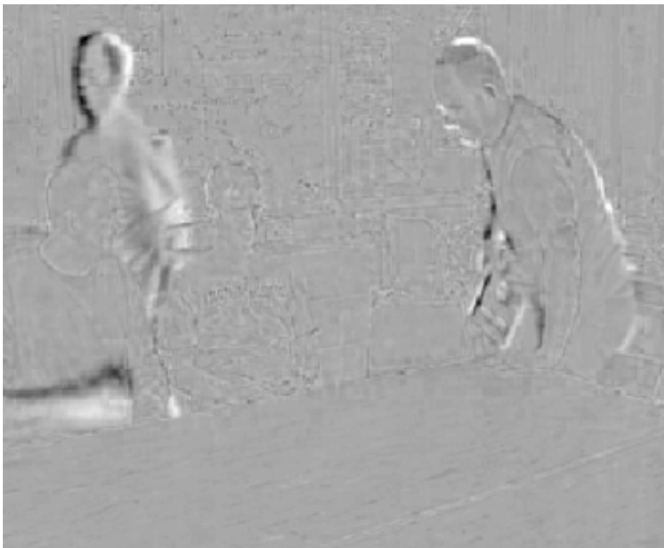
Fig. 3 Residual : no motion compensation
