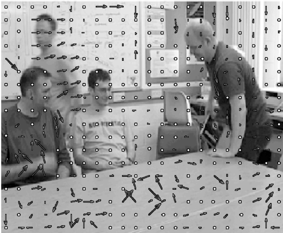
Fig. 4 16x16 motion vectors superimposed on frame
