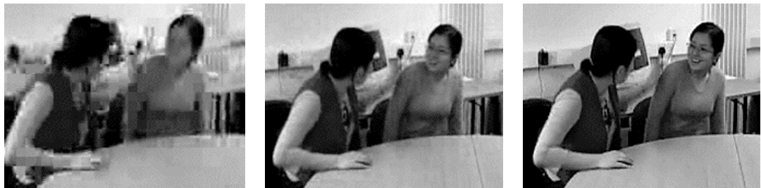
Figure 5 A video frame compressed at the same bitrate using MPEG-2 (left), MPEG-4 Visual (centre) and H.264 compression (right)
